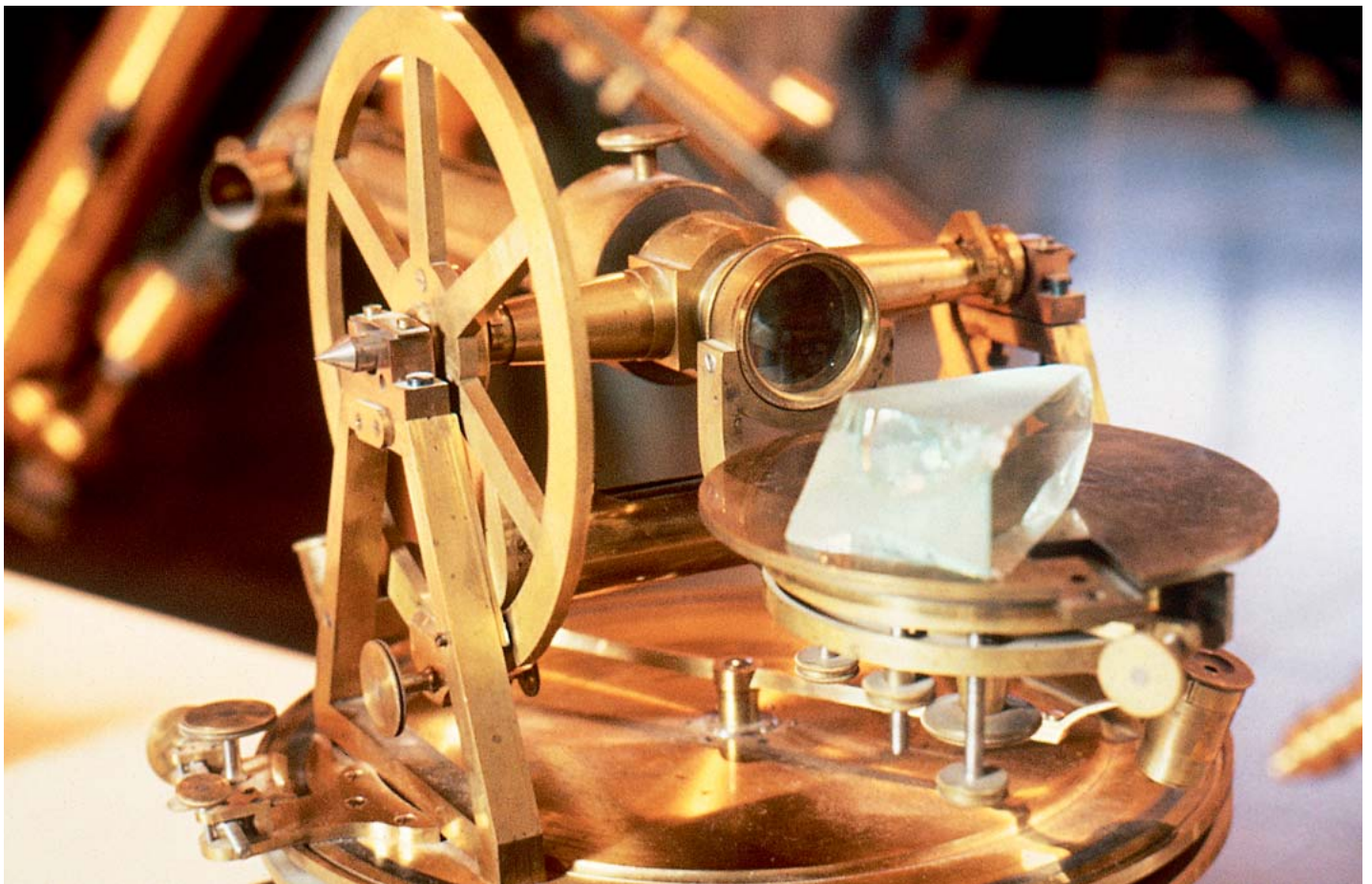
Spectral prism device from Fraunhofer's workshop. Such devices were used to separate the incident light into different wavelengths.
